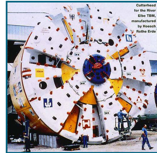
Elbe Tunnel Slurry Machine
